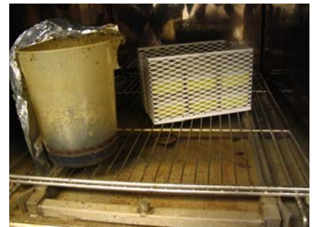
LIQUID RUN ON SOLIDS CYCLE— (NOTE BOIL-OVER IN CHAMBER FLOOR PLUS NO SECONDARY CONTAINER)
